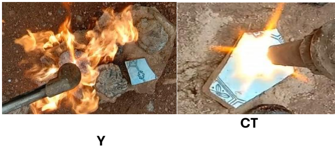
Figure 5. Flammability tests on the prepared polyethene composite tile (CT) and the conventional tile (Y).
