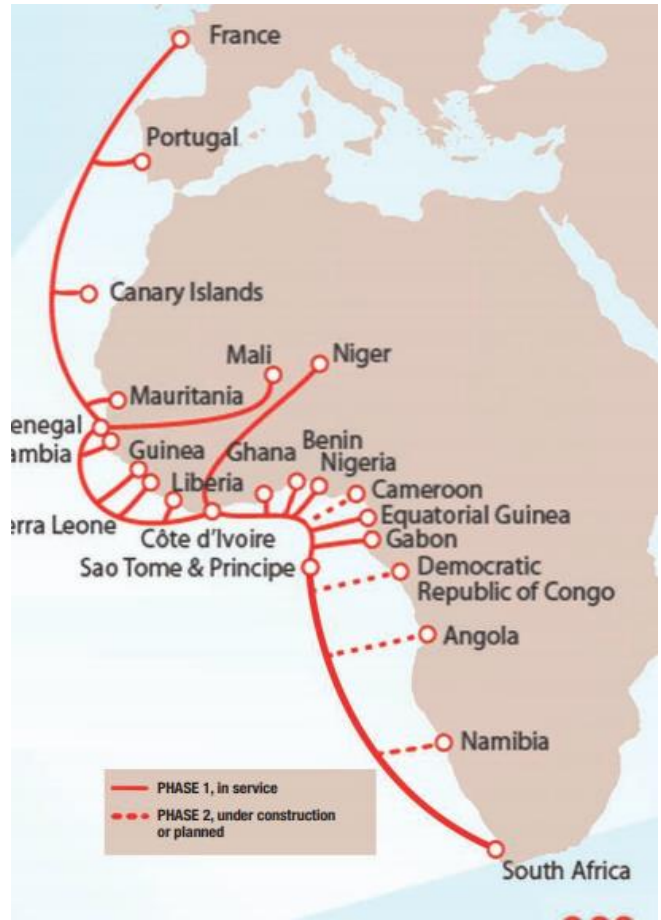
Figure 2: ACE: 17,000km long broadband optical submarine cable between Africa and Europe
